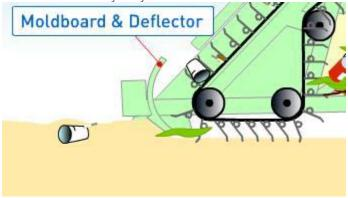
The moldboard performs several critical functions. It primarily:
