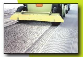
The nine foot wide, UV protected polyurethane groomer is attached to the SURF RAKE® with corrosion resistant, hot dip galvanized and stainless steel connecting hardware. The SURF RAKE® Finisher provides supreme value to any beach cleaning operation with appreciation from beach patrons to beach maintenance staff.
