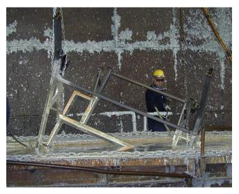
Following extensive preparation, the entire steel frame of the machine is immersed in molten zinc creating a tough protective coating, which is metallurgically bonded to the steel.
