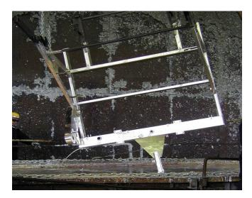
Following galvanization the frame receives a high quality industrial paint for a final layer of protection.
