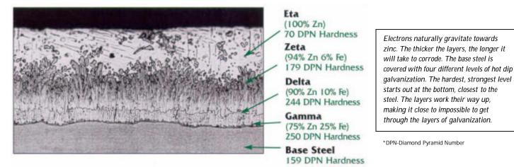
HOT-Really hot! At 800 degrees Fahrenheit, molten zinc metallurgically bonds to the base steel. The layers that are formed with the steel (called iron zinc alloys) are actually harder than the base steel itself! BASE STEEL AND THE MOLTEN ZINC MUST BE AT A MINIMUM OF 800 DEGREES FAHRENHEIT OR THIS BOND CANNOT OCCUR.
