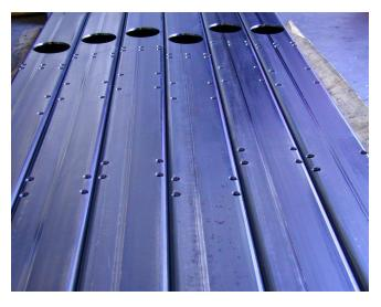
Preparatory holes are drilled into the frame allowing the molten zinc to flow inside the steel frame to coat and protect the frame both inside and out.
